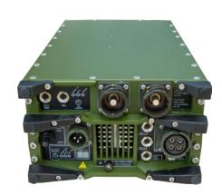
Introducing the unique ComPact 1200 Dual Input AC/DC & DC/DC power supply. Our advanced technology enables seamless switching between AC and DC input power sources, delivering consistent DC output. When AC input is available, it can provide clean 24V to your equipment while simultaneously charging the 12V battery connected to the DC input. Dual Input models are also available with 24 VDC and 36 VDC input.
