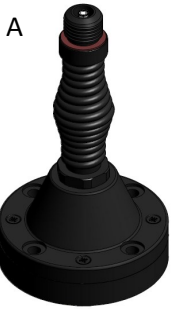
A NATO 4-hole Spring GPS Option 4 x M10 or 3/8" Bolts on 114mm (4.5in) PCD Base Dia. 140mm (5.5in)
