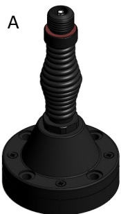
NATO 4-hole 4 x M10 or 3/8" Bolts on 114mm (4.5in) PCD Base diameter 140mm (5.5in)
